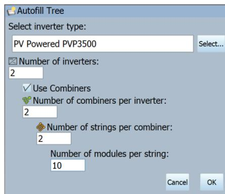
**Figure 56. Autofill tree screen**
