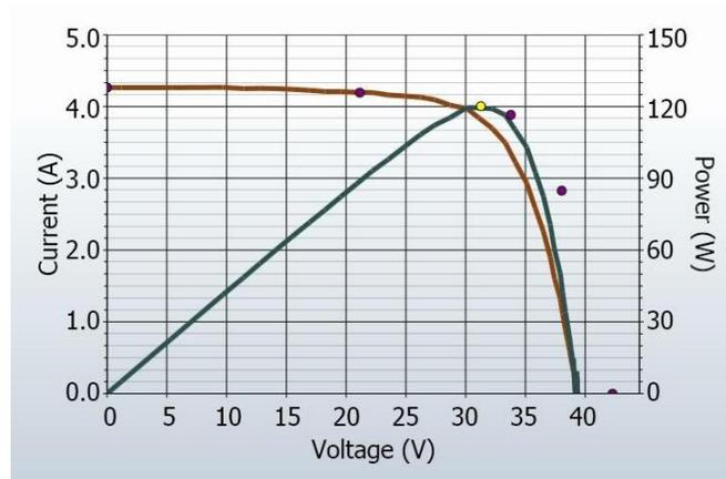
**Figure 69. Measurement with less steep than predicted slope in the vertical leg of the I-V curve.**
