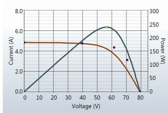
**Figure 72. Measurement with less steep slope in the vertical leg of the I-V curve.**
