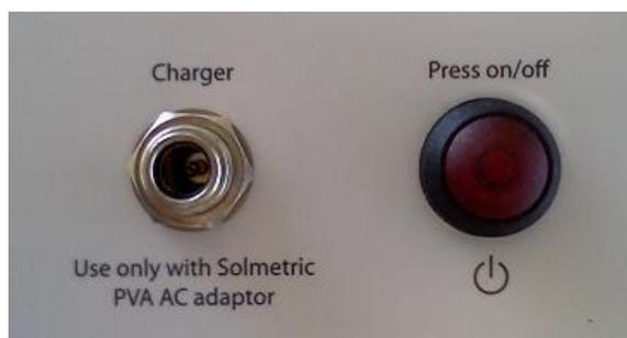
**Figure 11. Battery charger connector on the I-V Unit**
