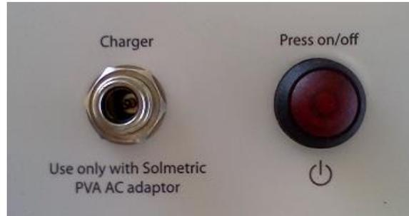
**Figure 25. Powering-up the I-V Unit**
