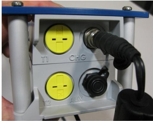
**Figure 12. Charger connected**
