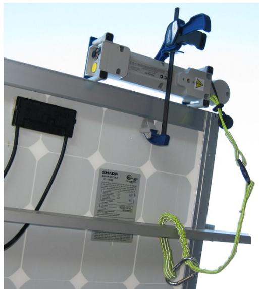
**Figure 17. SolSensor's tool lanyard secured to a racking member.**
