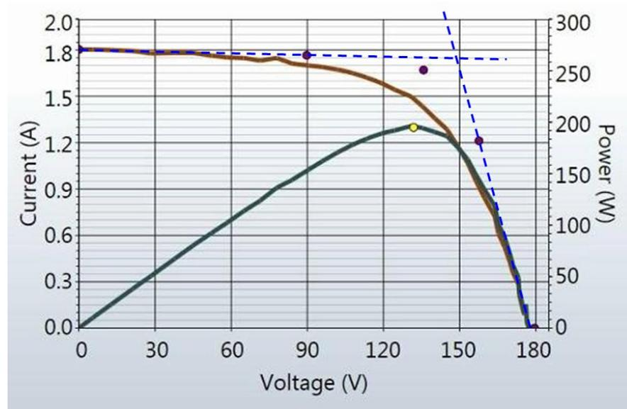
**Figure 70. I-V curve measurement showing rounder knee than predicted by the PV model.**
