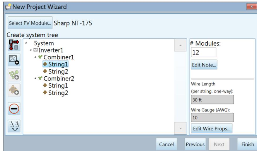
Figure 34. Array Navigator Screen with Example System Tree
