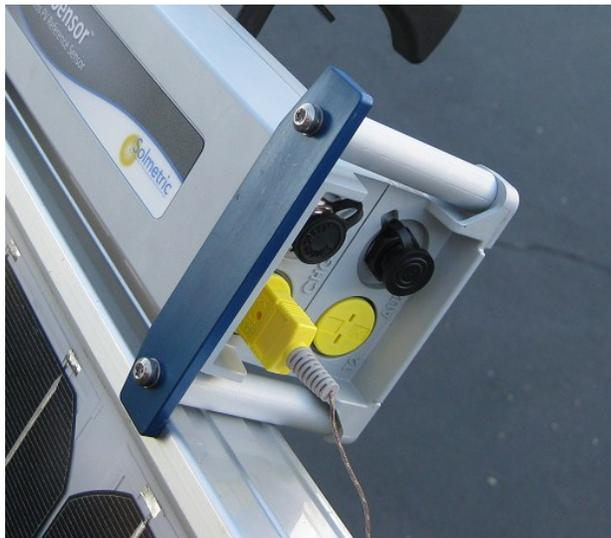
**Figure 20. Thermocouple plugged into the TC1 connector.**
