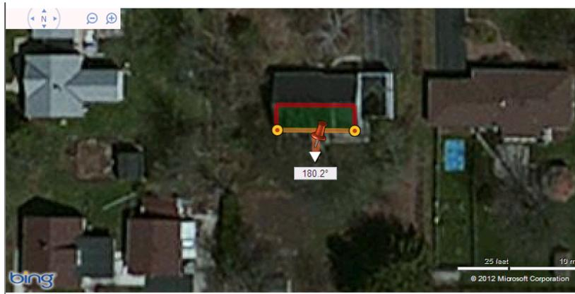
**Figure 52. Measuring your roof orientation**
