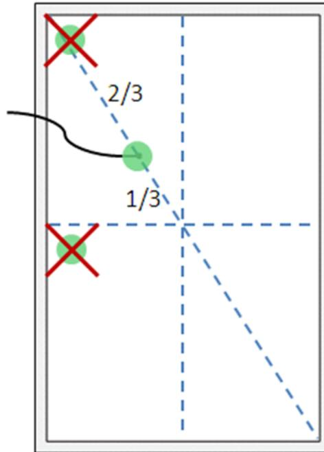
**Figure 21. Locating the thermocouple tip on a single free-standing module.**
