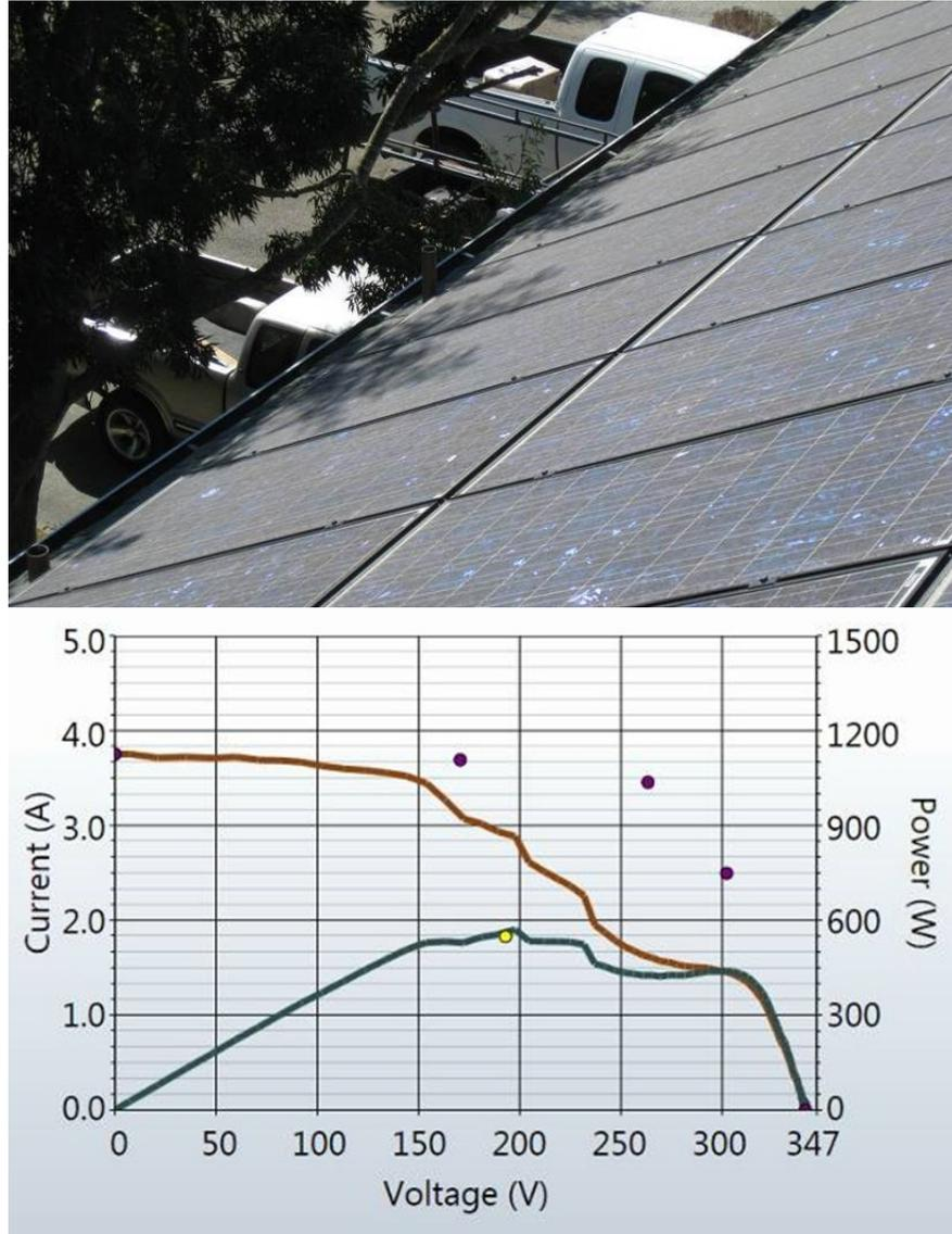
Figure 66. The effect of partial shading on a string I-V curve.
