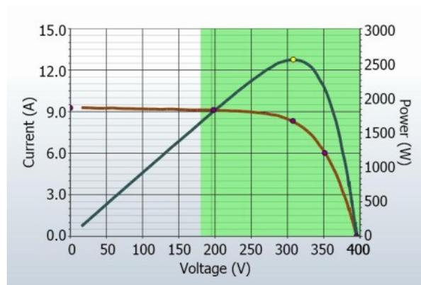
**Figure 64. A normal I-V curve for the parallel combination of two strings of eight 175-watt modules, showing conformance with five points predicted by the PV model.**
