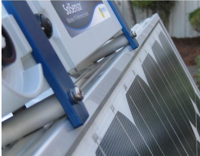
**Figure 18. SolSensor correctly seated along the upper horizontal leg of the module frame.**
