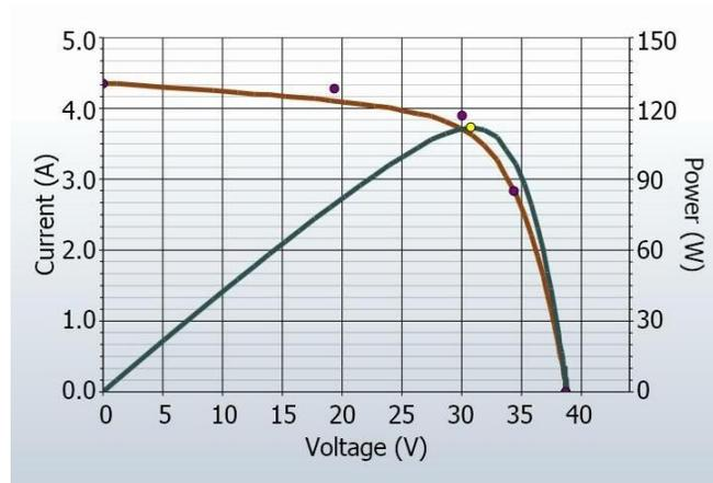
**Figure 71. An I-V curve showing steeper slope in the horizontal leg of the I-V curve.**
