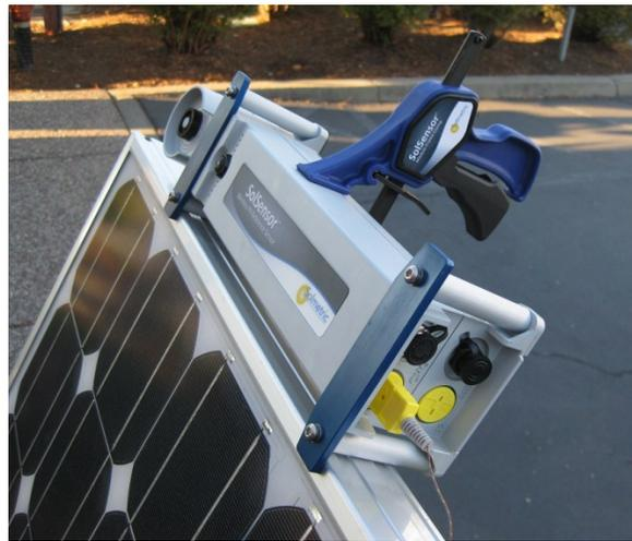
**Figure 16. SolSensor mounted along the upper frame edge of a PV module**
