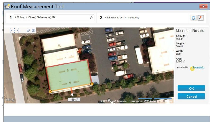
**Figure 31. Finding the Azimuth Value Using the Roof Measurement Tool**
