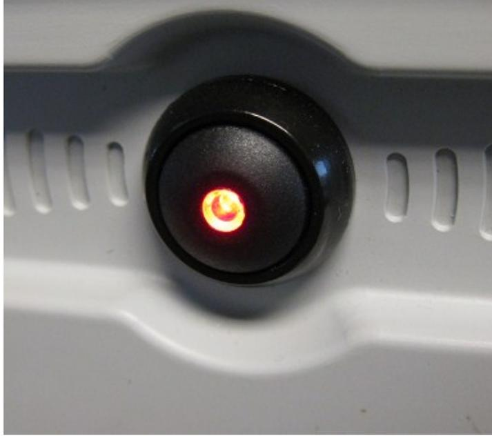
**Figure 22. Pushbutton with LED lit. LED blinks until wireless network is established, after which it remains on.**
